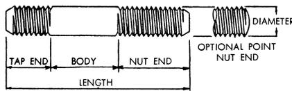
Tap-end studs have a short thread on one end called the tap end which is threaded to a Class NC5 or Class UNRC-3A fit. This end is for screwing into a tapped hole. The other or nut end is threaded with a Class UNRC-2A fit. Length of the stud is measured overall. The tap end has a chamfered point, but the nut end may have either a chamfered or round point, at the manufacturer's option. Tap-end studs are available in four types, as follows:
