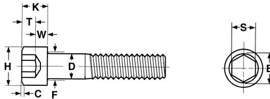
METRIC - SOCKET HEAD CAP SCREWS, CLASS 12.9
