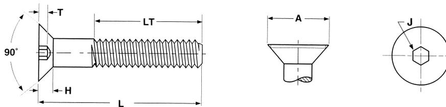
METRIC - FLAT HEAD SOCKET CAP SCREWS, CLASS 10.9
