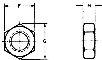
**Heavy Hex Jam Nut, washer-faced and double-chamfered**
