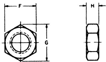
**Hex Jam Nut, double-chamfered**
