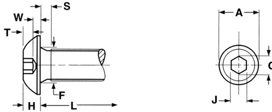
METRIC - BUTTON HEAD SOCKET CAP SCREWS, CLASS 10.9
