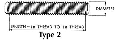
Continuous-thread studs are threaded from end to end and are often used for flange bolting with two nuts applied.
